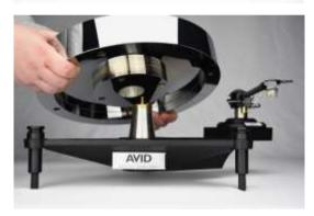
Gently and gradually place the platter onto the main bearing, ensuring that the spindle does not come into contact with or leave any scratches on the tapered bore in the platter.
