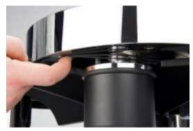
With a gentle touch, lift the platter edge to expose the motor pulley. Rotate the platter to engage the belts with the grooves of the drive pulley. Using your finger, hold the drive belts against the underside rim of the platter, and then remove the fitting pin. Finally, let go of the drive belts, and they will be secured in place.
